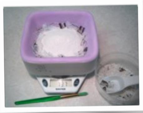
Carefully layer the frit mixture into the mold on top of the white frit mixture. The mixture should be slightly mounded. When casting with large frit, billets, or sheet glass, hot glass pieces drag down the mold's interior sidewalls as they melt and compact. This action may cause glass spurs to develop on the piece's perimeter. Mounding the frit towards the mold's center reduces glass spurs along casting's perimeter.
