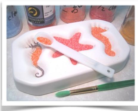
To make our samples, we used fine mesh frit. Further, we mixed our frit colors with equal amounts of fine clear frit. The results were
