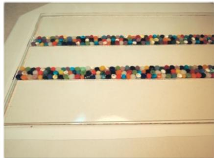
After the panel has cooled, transfer the panel to the prepared slumping form. Fire according to the Slumping Schedule.
