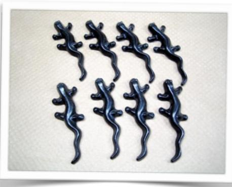
either Hotline Primo Primer or ZYP BN Lubriccoat Aerosol (formerly MR-97). If you are using Hotline Primo Primer, give each mold four *thin*, even coats. It is the only traditional primer we recommend because it doesn't obscure the mold's fine detail and is easy to remove after firing. Use a soft brush to apply the primer and
