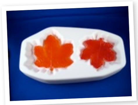
The next step is to slump the leaves using the slumping surface built into the Maple Leaves molds' reverse side. Just like mold's casting surfaces, the slumping surfaces need to be coated with primer. Follow the instructions in the previous paragraphs to apply four to five,
