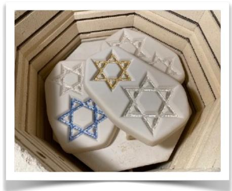
Fill the remainder of each cavity with the specified medium Clear frit. Evenly distribute it and, if necessary, gently use the artists brush to level the Clear frit.
