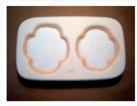
Place mold on elevated kiln shelf. Avoid thermal shock – breaking the mold – by heating mold no
