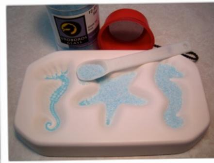
Remove any existing kiln wash using a stiff, nylon brush. Spray the mold with ZYP as described above, but using a two to three-second blast since the mold is smaller. Just as before, spray the mold twice if this is the first time
