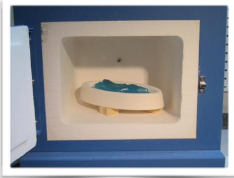
Fire the molds according to the Component Casting Schedule. The low temperatures of this schedule will preserve the designs' delicate edge detail and keep the
