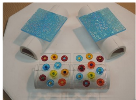
Panels Lined-up and Ready to Slump
