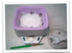
Carefully layer the frit mixture into the mold on top of the white frit mixture. The mixture should be slightly mounded. When casting with large frit, billets, or sheet glass, hot glass pieces drag down the mold's interior sidewalls as they melt and compact. This action may cause glass spurs to develop on the piece's perimeter. Mounding the frit towards the mold's center reduces glass spurs along casting's perimeter.
