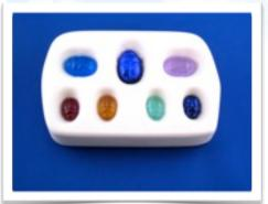
Medium frit (or a combination of medium frit colors) is a good choice to fill each scarab as it produces castings with fewer bubbles. Use a small brush to move any stray frit into place and level the surfaces. Fire according the attached schedule.
