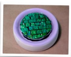
After the glue has dried, transfer the black disks into the primed lid mold. Cap the dichroic glass with the clear, glass disk.
