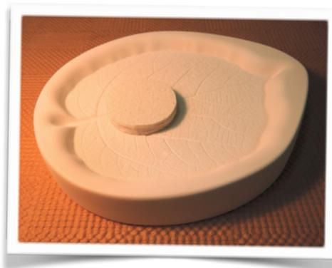
This plug is used to make a hole in the cast leaf. *Note: If  $\frac{1}{8}$ " fiber paper is not available, use a combination of other thickness to get the same results.*
