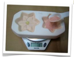
Use you scale to weigh out two 15 gram parcels and one 18 gram parcel of the green mixture. Place these mixtures in the three cavities of the Leaves (3) mold. Again use a brush and your fingertip to distribute and pack the frit. Move the filled molds to the kiln.
