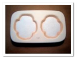
Place mold on elevated kiln shelf. Avoid thermal shock – breaking the mold – by heating mold no faster than 350°F per hour until 1250°F is reached.
